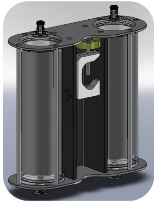
Dual Filter Housing with Integrated Pole Mount
